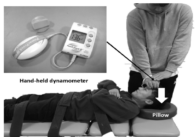
Figure 3. Neck flexion isometric strength measurement. White arrow represents the direction of the applied force
