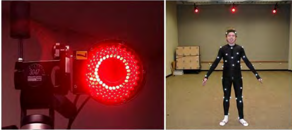
Fig.9.c.d, Infrared camera for motion analysis and markers on the subject
